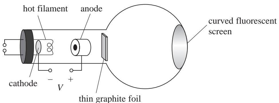
The potential difference,  $V$ , accelerates electrons from the hot filament towards the thin graphite foil.
